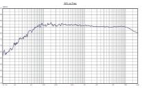
Figure 1: Pink noise frequency response at one watt at one metre.
